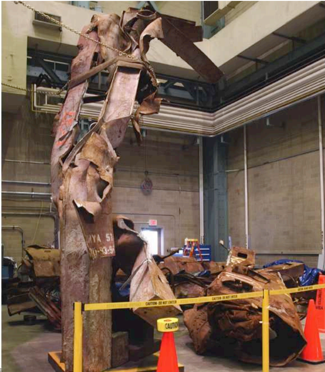
WTC steel recovered from the point of aircraft impact. Source: NIST
