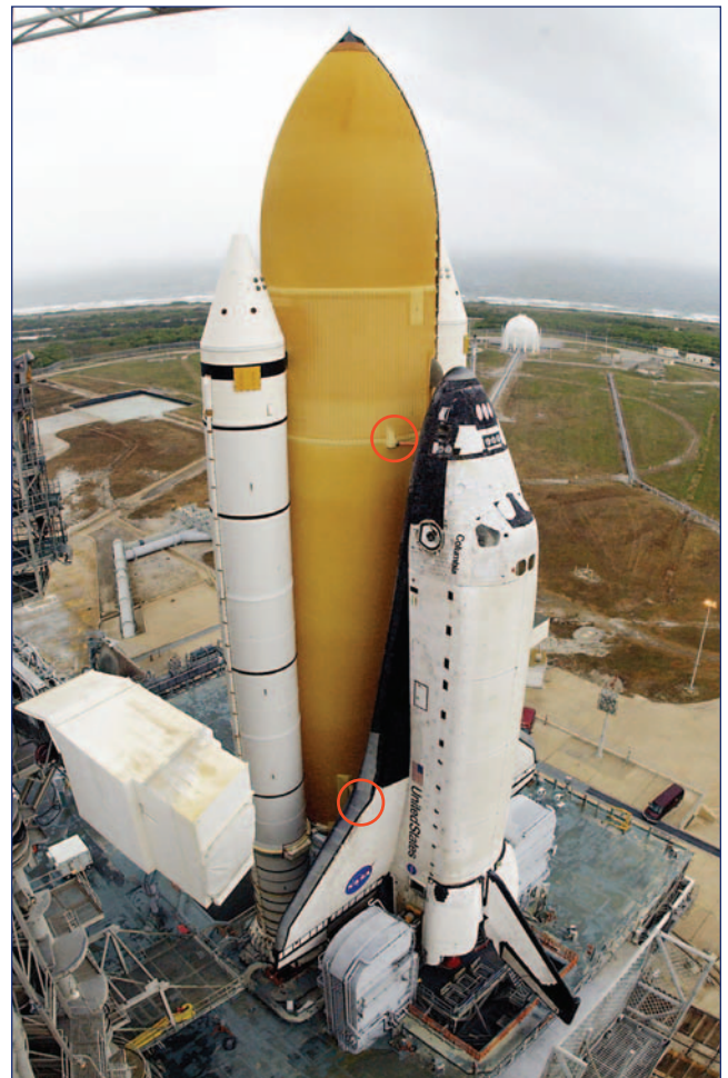
Figure 3.1-1. Columbia sitting at Launch Complex 39-A. The upper circle shows the left bipod (-Y) ramp on the forward attach point, while the lower circle is around RCC panel 8-left.
