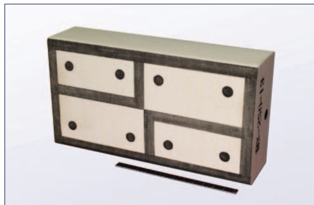
Figure 3.8-3. A typical foam projectile, which has marks for determining position and velocity as well as blacked-out outlines for indicating the impact footprint.
